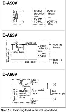
Note 2) Wiring to the load is 5 m or longer. Note 3) Load voltage is 100 VAC.
